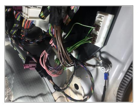
Connect black wire from alarm (ground) to chassis ground
