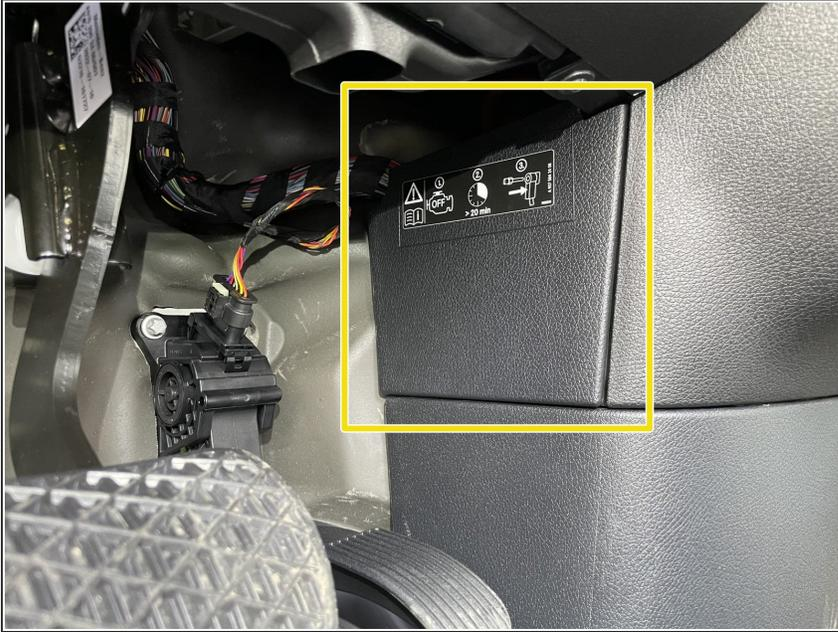
**i** There is a battery quick disconnect that should be used to disconnect the chassis battery ground before performing this bypass
