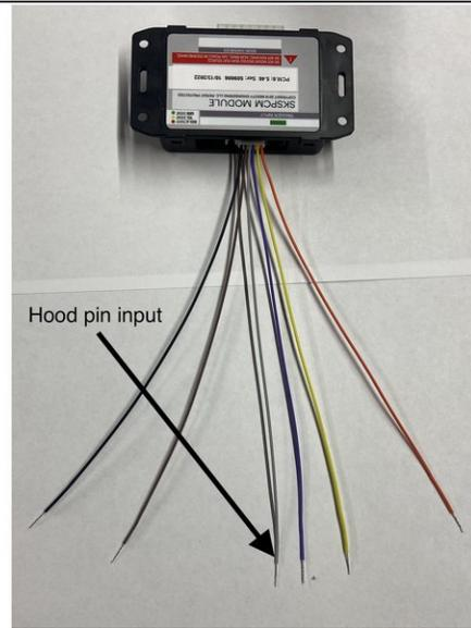
**!** Run wire from hood pin securely through firewall and run to driver side under dash area
