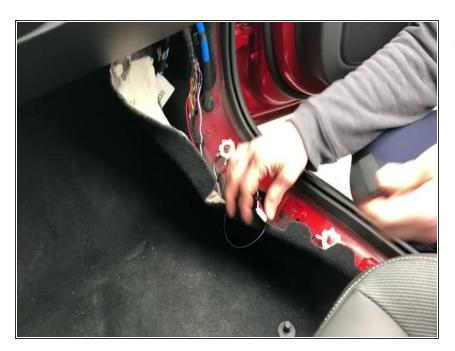
Plug SKSXC module into SKSXC wiring harness
