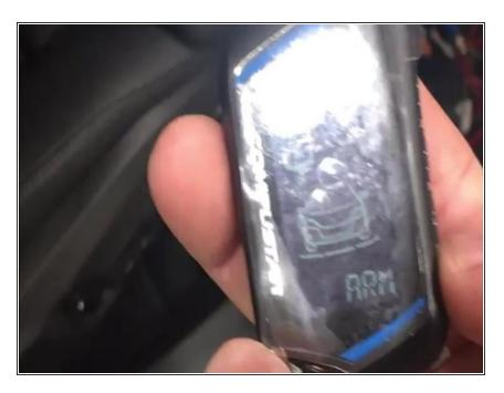
Once RF remotes are programmed (see previous step), test remote start/stop, lock/unlock from external RF remotes
