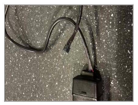
Plug Compustar Drone into grey port on SKSXC module
