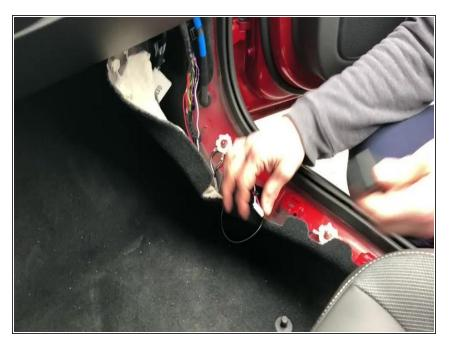
• Plug SKSXC module into SKSXC wiring harness
