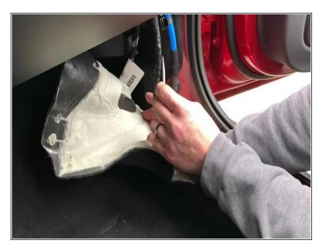
Cut section of tape and remove so that wires in harness can be accessed
