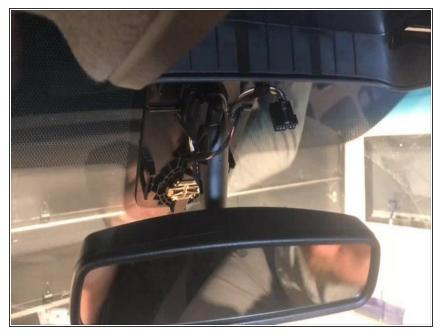
Plug black 6 pin factory camera cable into 6 pin socket on 907CAM harness
