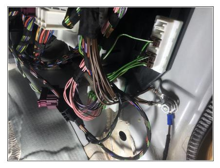
Connect black wire from alarm (located in 6 pin low-current harness) to chassis ground
