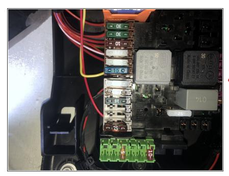
Connect red wire from alarm brain (located in 6 pin low-current harness) to constant power at fuse box (red wire)
