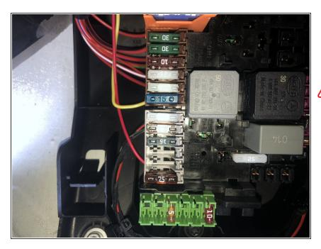
Connect green ignition wire from alarm brain (in 6 pin plug) to ignition source at fuse box
