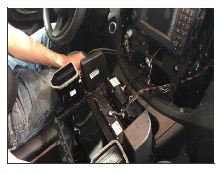
Replace bezel and vents around radio and clip into place
