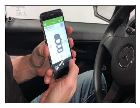
Using Compustar Drone app, test lock, unlock and start controls
