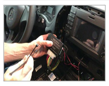
Use zip ties to mount key box module and NG module together
