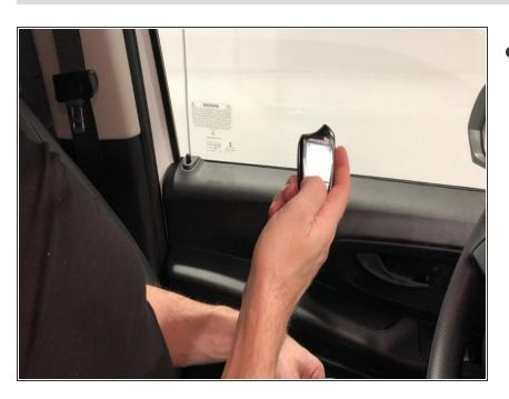
Using Compustar RF fob, test lock, unlock and start controls
