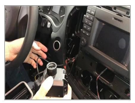
Route EIS through left side of radio cavity and into dash
