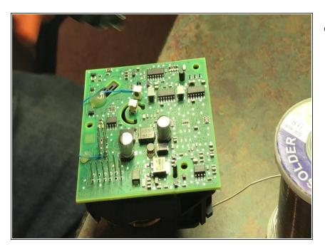
Apply glue and adhere cable in place on board of EIS
