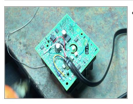
Use additional glue to secure wires to board
