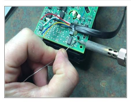
Add solder to contacts where cable will be connected to board of EIS
