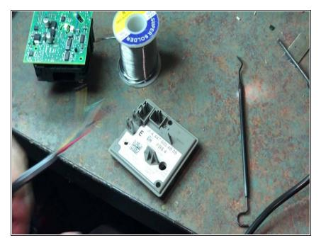
Route bare end of cable through hole drilled in previous step. The bare wires will be connected to board
