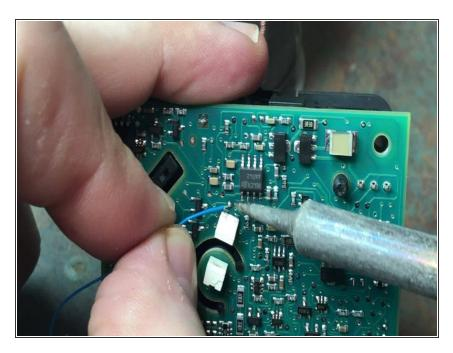
Solder other end of wire to contact where solder was added near optical sensor in step 3
