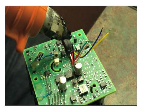
Put additional glue on top of cable to further secure in place
