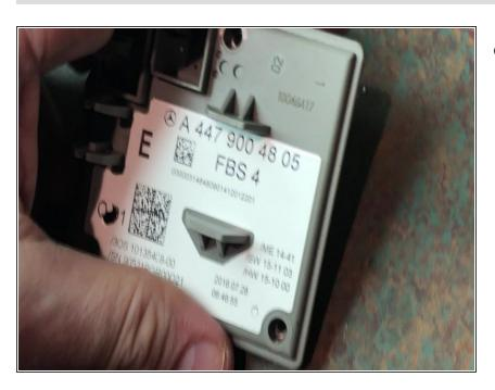
Drill hole in rear cover of EIS to route cable
