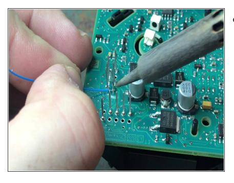
Attach wire to pin that was inserted in last step
