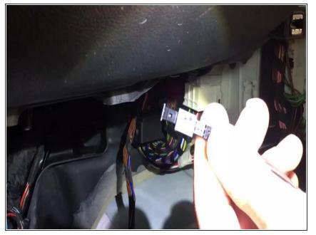
Remove adapter from end of provided CAN plug. Factory CAN wires will be pinned into this plug
