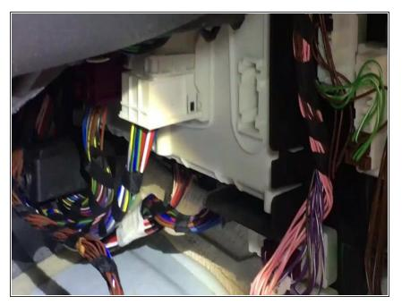
Plug factory CAN B plug back into front SAM module
