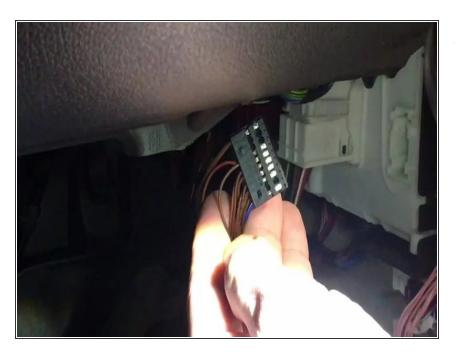
Using pick tool, carefully remove brown (pin 7) and brown/red (pin 17) wires from CAN B plug
