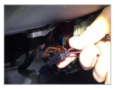
Slide factory shroud over CAN B plug so that it can be plugged into the SAM module
