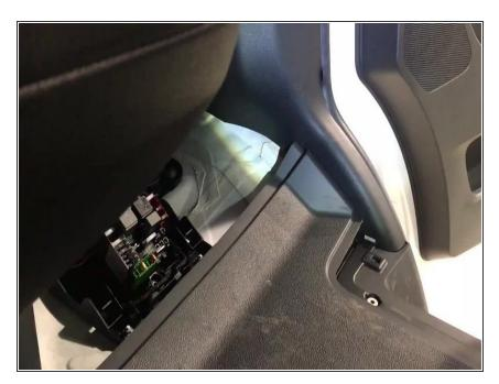
Pull back floor and remove sill panel
