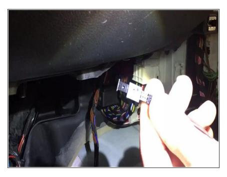
Remove adapter from end of provided CAN plug. Factory CAN wires will be pinned into this plug
