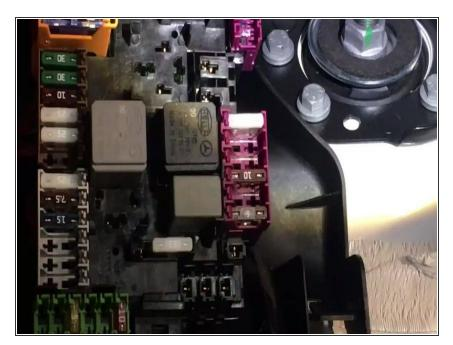
Pin provided fuse terminal on red wire into open spot shown in video
