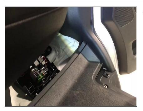
Pull back floor and remove sill panel
