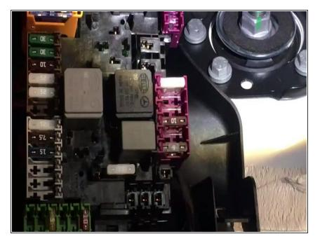
Pin provided fuse terminal on red wire into open spot shown in video
