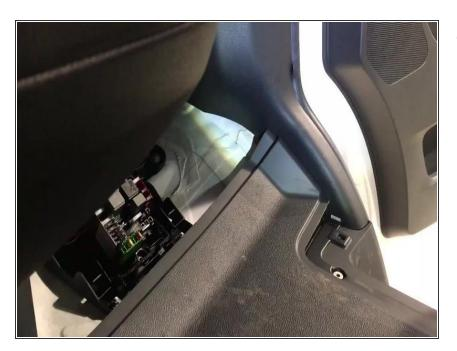
Pull back floor and remove sill panel
