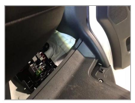
Pull back floor and remove sill panel
