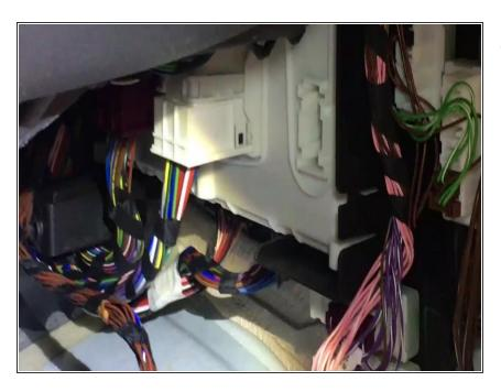
Plug factory CAN B plug back into front SAM module
