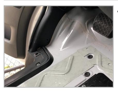
Remove 1 x T25 screw from panel below A pillar
