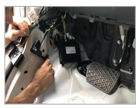
Place and clip PCM module back into bracket
