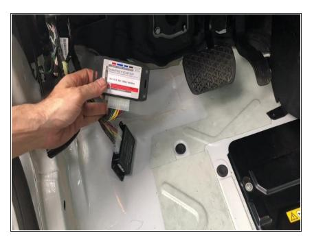
Connect white 2 pin plug from key box into port labeled 'KEY' on SKSNG module (labeled SMARTKEY STARTER)
