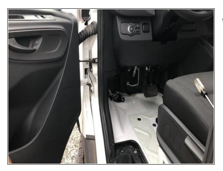
Pull back weather seal from driver door jam
