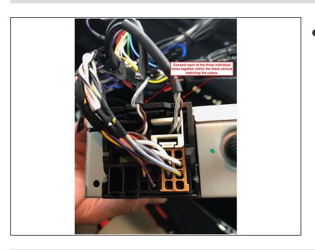
There are 2 cables with a black casing that enter the radio harness. Each casing houses (3) wires. Those wires need to be connected together, individually, matching the colors, in order for the S.O.S. microphone to be able to continue communicating with the system without the original radio present.
