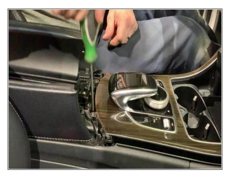
Remove 2 screws from under center console trim piece
