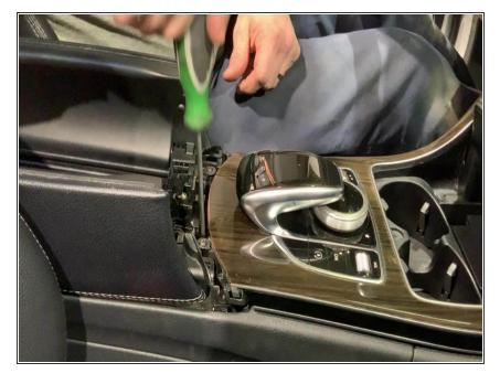
Remove 2X T-20 screws in front of center console
