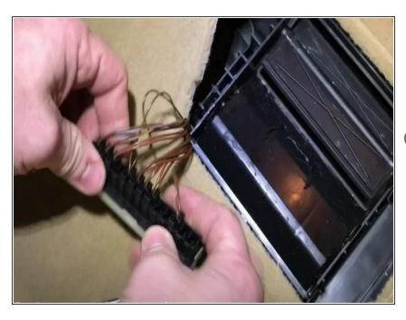
i To find the KG CAN plug, you will un-plug the connectors from the distribution block with brown and brown/red wires one at a time and observing the LED on the SKSNG205D4 module. When the KG connector is un-plugged, the yellow LED on the SKSNG205D4 module will shut off.
