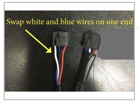
An RS232 cable is used to connect the Compustar alarm to the SmartKey Starter®. The RX and TX wires (white and blue) must be opposite on each end. Most cables will need to have the RX and TX wires reversed on one end of the cable.
