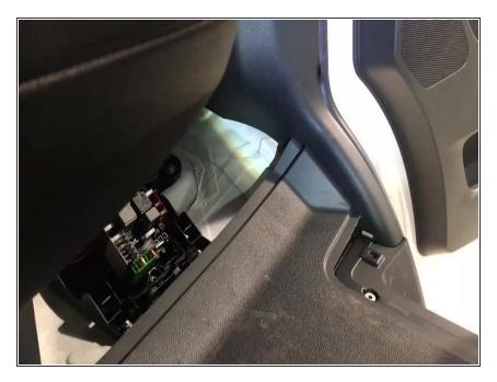
Pull back floor and remove sill panel
