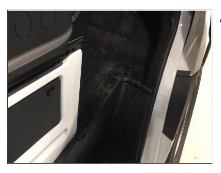
Remove two screws and panel and end of footwell
