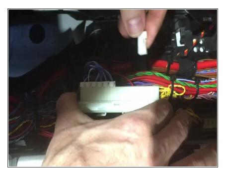
Connect 2 pin white plug from provided T-harness (side without exposed pins) into any empty spot in the block
