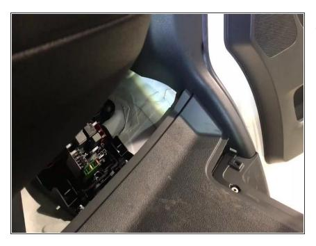
Pull back floor and remove sill panel
