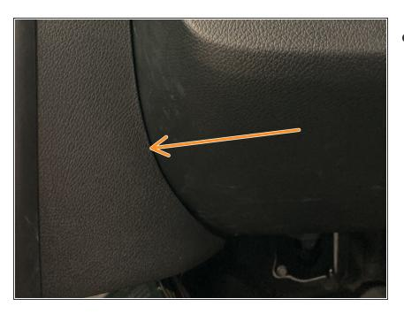
Using a pry tool, remove panel between A pillar and kick panel.
