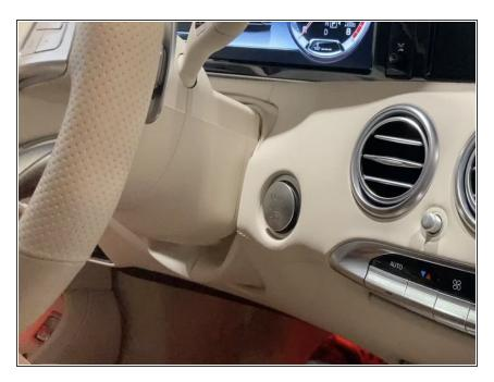
Turn ignition on (without starting, by pressing the push button 2X (without foot on brake). Or insert key and turn to 2nd position
