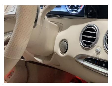
Turn ignition on (without starting) by pressing the push to start button 2X (without foot on brake) or inserting key and turning to the 2nd position
