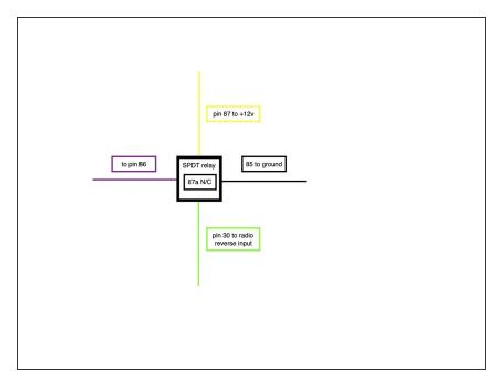
Any 12v SPDT relay can be installed at the end of the purple lead in the 907CAM harness. The output from the relay will go to the radio reverse trigger as shown
